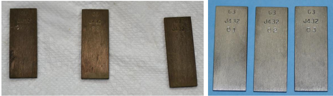
Figure 5. Alloy G3 after testing in 50%vol Oil Safe AR® at 420°F before (left) and after (right) glass bead blasting.
