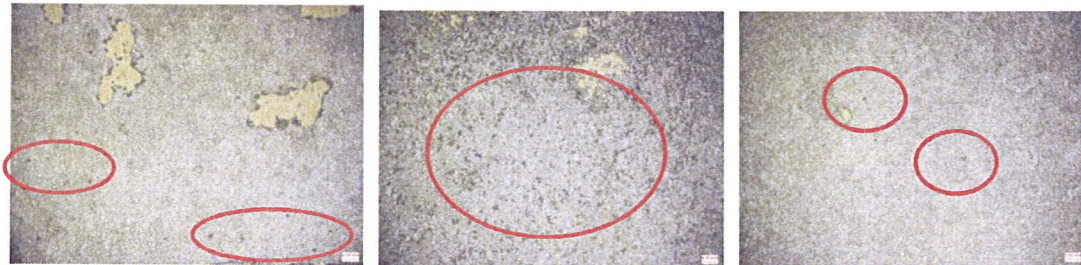
Figure 3. Slight pitting on carbon steel coiled tubing samples after testing in 50%vol Oil Safe AR® at 420°F for 24 hours. Original magnification at 20X.
